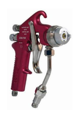
Medium pressure spray gun with airless atomization and additional air for fan adjustment and uniformity of spraying. Practical, handy, soft in product distension. Ideal for use with pressures from 80 to 120 bar.
